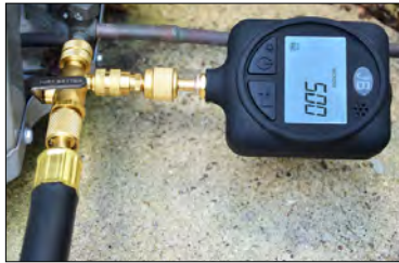
Easily attaches and protects vacuum gauge with the slide valve side port
